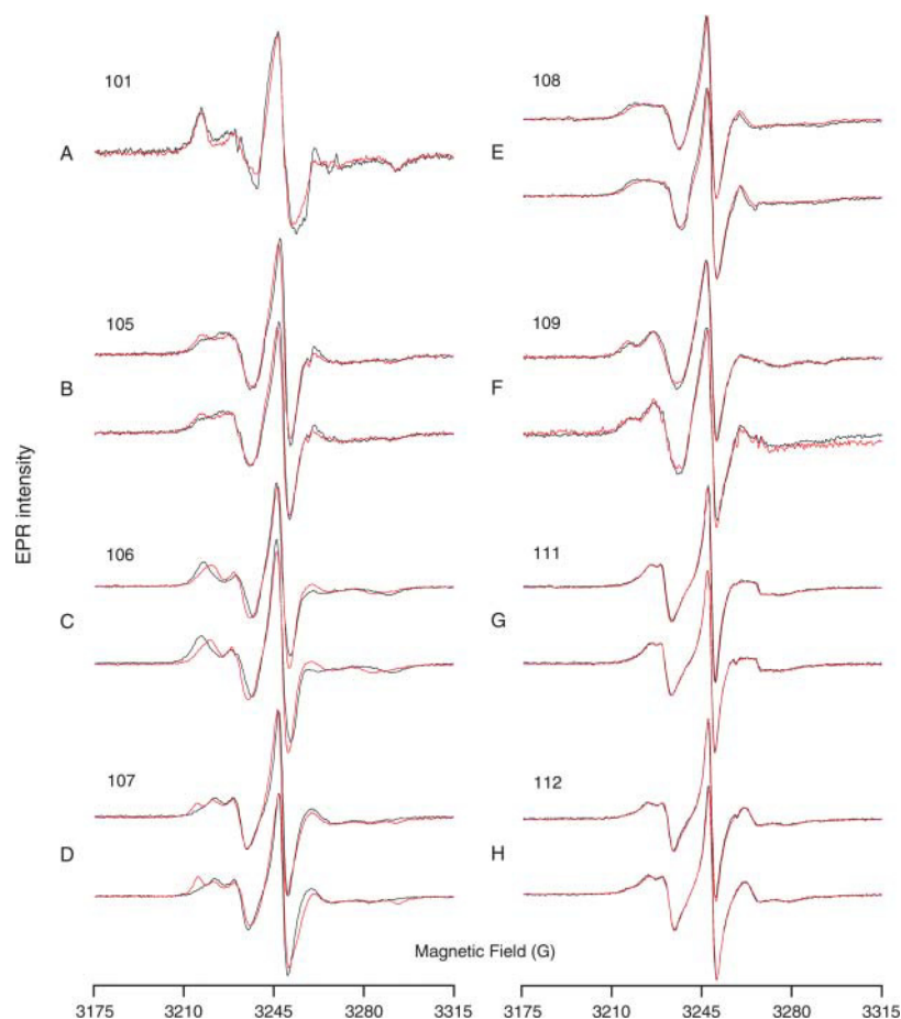
FIGURE 3 EPR spectra of spin-labeled ERK2. Spectra corrected for free probe are shown, corresponding to sites labeled at positions (A) 101, (B) 105, (C) 106, (D) 107, (E) 108, (F) 109, (G) 111, and (H) 112 of unphosphorylated (black) and diphosphorylated (red) ERK2. Spectra obtained from independent protein preparations and labeling reactions are shown to illustrate the reproducibility of the experiment.
